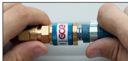
3. Mounting is finished. O-ring is visible.
