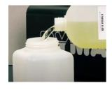
Now, add some electrolyte to the wide-neck container, being careful not to spill anything. Do not leave the brush in the container, as it may tip due to the weight of the handle.
