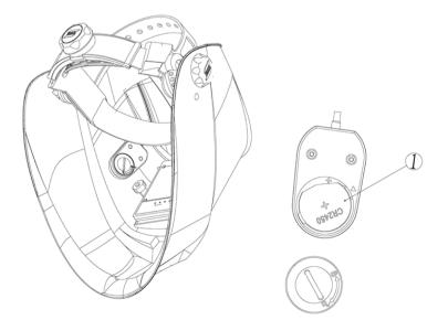
3) Assemble battery cover onto battery case.
