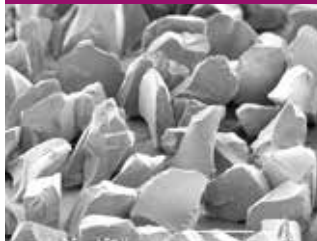
Conventional ceramic grain is irregular and 'ploughs' through the metal.
