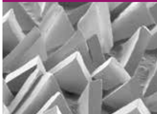
Precision-Shaped Ceramic Grain slices cleaner and faster.
