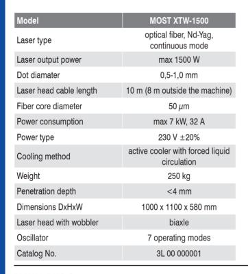
MOST XTW-1500 laser welding machine is a set which includes:
