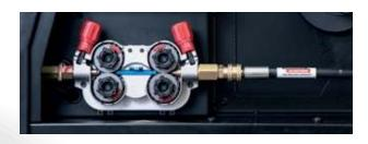
Connection for drum feed (optional adapter). Less need to change wire spools saves time
