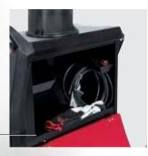
Practical, big storage locker inside the power source with key lock, internal lights, for accessories like gun, gloves, rolls, contact tips, etc.
