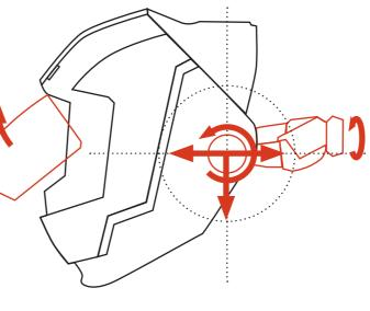
Outer front cover made of robust injection moulding with innovative quick-release fastener:
