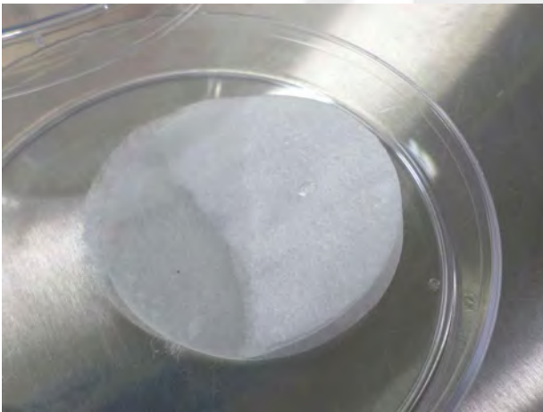
Photo 1. Control textile demonstrating hydrophobicity on one portion of the prepared carrier. Despite this full absorption of the viral inoculum was achieved by recovering un-absorbed inoculum and re-inoculating absorbent portions of the product.
